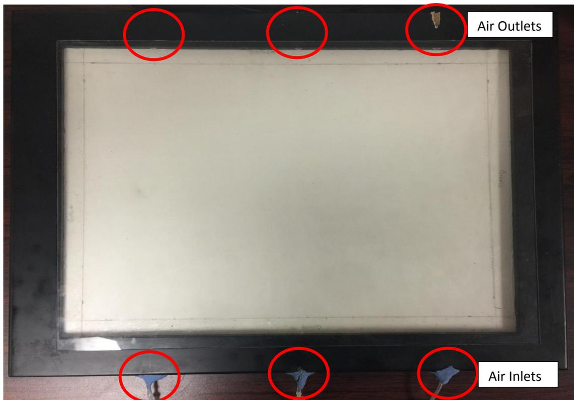
**Figure 1. A top view of the test arena showing the three evenly spaced parallel inlet and outlet air holes circled in red. Air would flow through each area in the arena with minimal mixing at  $0.2\text{L}\cdot\text{min}^{-1}$ .  $0.2\text{L}\cdot\text{min}^{-1}$  was the maximal air flow before there would be turbulent flow through the arena. Inlet holes were 6mm in diameter while outlet holes were 8mm in diameter to help reduce resistance to airflow.**
