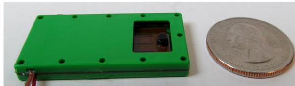
Figure 4. SHIVR™ ST-25b piezoceramic tactile stimulator (quarter for reference).
