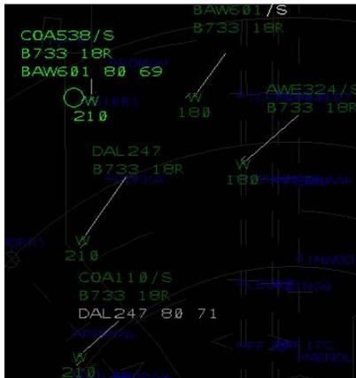
**Figure 3:** Controller Display with merging and spacing tools.
