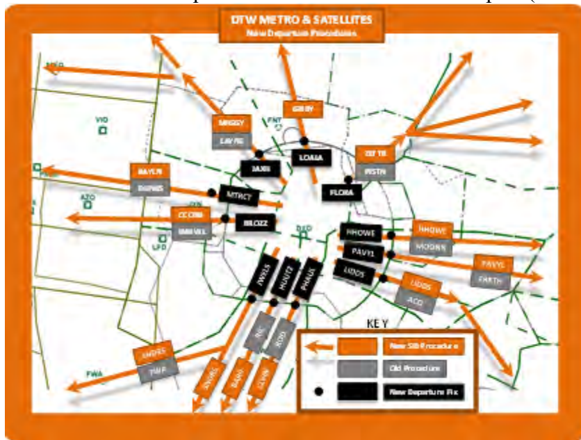
Figure 1. RNAV SIDS for departures out of DTW.
