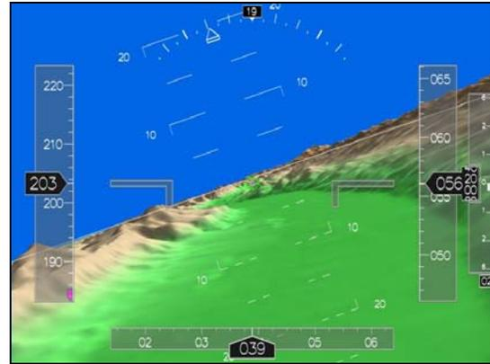
**Figure 2.** Synthetic Vision System (SVS).
