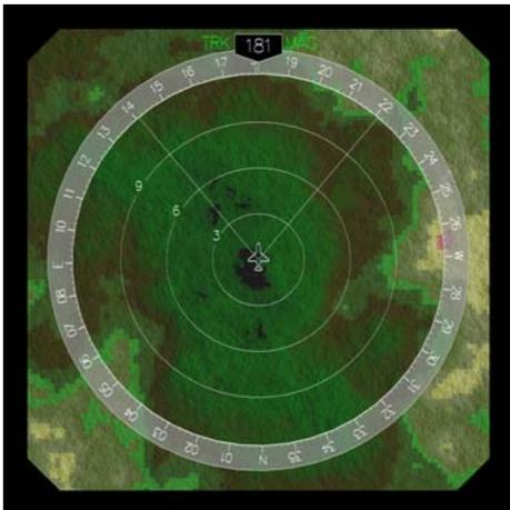
**Figure 1.** Terrain awareness display of the Enhanced Ground Proximity Warning System.
