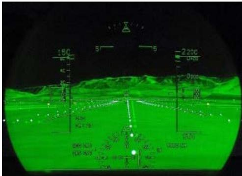
New vision systems that are available for use by the pilot, and which are the subject of FAA human factors research, include advanced vision systems permitting low-visibility taxi and takeoff operations. The FAA is also studying enhanced flight vision systems that allow landing at airports with reduced airport infrastructure. Other areas of research focus on determining minimum requirements with synthetic vision and combined vision systems.
