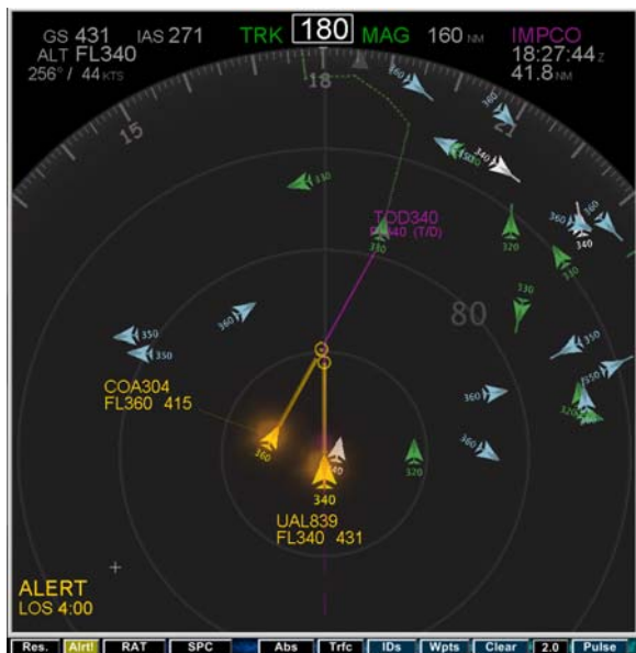
Figure 3. CDTI showing an SA3 alert level. Alert button lights up in yellow (bottom, second from left).
