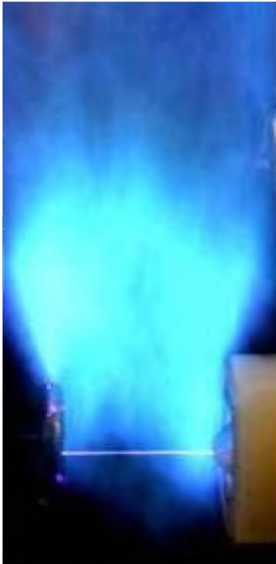
Experiments conducted to test capability to breakdown air and ignite fuel at various electrode gaps and applied voltages
