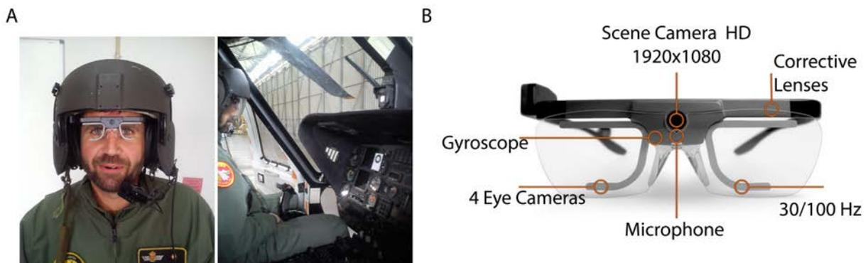
**Figure 2.** A) Left. A flight instructor from the Spanish Air Force Helicopter School (78th Air Base Wing) (Armilla, Spain), wearing his helicopter flight helmet and the eye tracker. Right. Calibration procedure inside a Sikorsky S-76 helicopter using a single point calibration. B) Tobii Pro Glasses 2.0 and its technical details.
