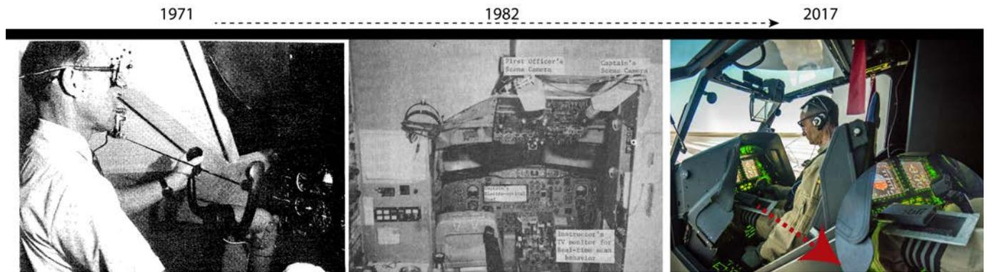
**Figure 1.** Advances in eye tracking technology in aviation settings. From left to right: **1971)** Eye Point-of-Regard System mounted in an eyeglass frame (Source: Weir & Klein, 1971). **1982)** Honeywell electro-optic head (Source: Harris, Glover, & Spady, 1986). **2017)** Tobii Pro Glasses 2.0 and its recorder unit (attached to the pilot’s kneeboard) (Source: Diaz-Piedra, Catena, et al., 2016).
