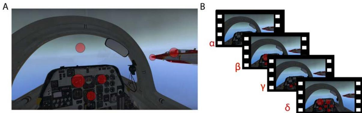
**Figure 4.** OT<sup>3</sup>: *augmented videos*. A sketch of our OT<sup>3</sup> showing different frames of an augmented video. These videos contain the trainee pilot's eye movements superimposed onto the first-person perspective video captured by the integrated scene camera. Also, the communications between the flight instructor and the trainee pilot are recorded. Flight instructors can use these videos to point out accurate and mistaken maneuvers in debriefing sessions.
