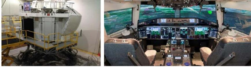
Figure 1. Research Flight Deck Simulator
