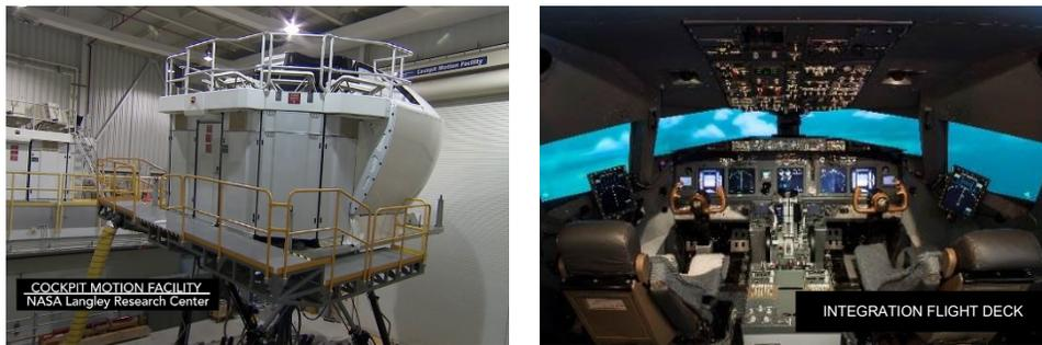
Figure 1. NASA 737-800 High-Fidelity Full-Motion Simulator
