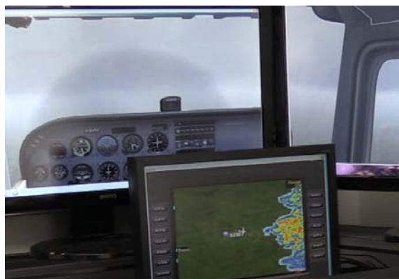
Figure 1. The weather radar image on the portable device screen shows a better weather situation that existed earlier at the aircraft current position.
