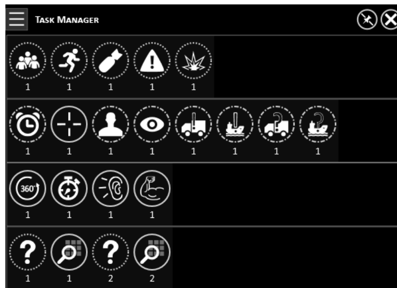
Figure 4. The left pane of Task Manager showing agent generated tasks in four rows, each row decreasing in priority. The following identifies the mission tasks, from left to right, for each row. Row 1: crowd forming, gate runner, mortar fire, perimeter breach, explosive device. Row 2: building/fence alarm, overwatch (provide air coverage), escort, eyes on (location), suspicious vehicle/watercraft, unidentified vehicle/watercraft. Row 3: 360 check, interval (temporal) check, listening post, and show of force. Row 4: queries and information retrievals (two each).
