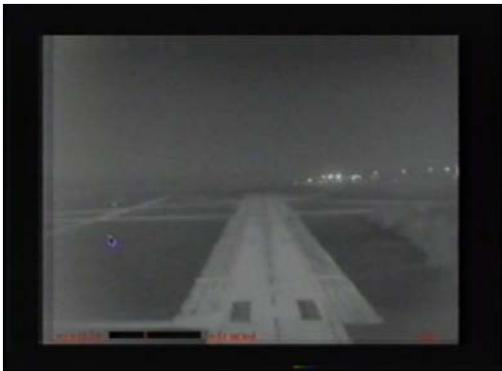
**Figure 1.** A picture of the EVS display that combines both infra-red and light intensification technologies.
