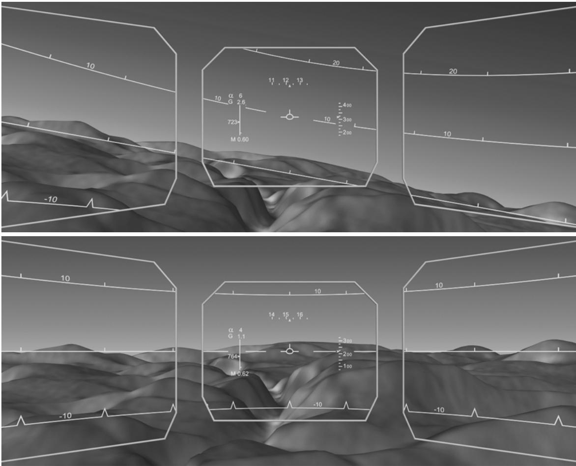
**Figure 3.** The Gripen HUD concept applied to one version of a wide FOV interface design. The illustrations show horizontal flight at the bottom, and a roll position in a pitch attitude above horizontal at the top.
