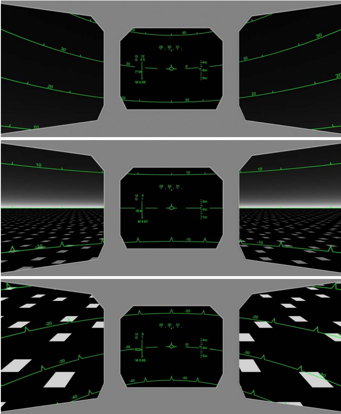
**Figure 4.** An illustration of an IMC mode of the suggested interface with peripheral visual flow. The flight sequence from bottom to top: From pitch-down to pitch-up including horizontal flight in between.
