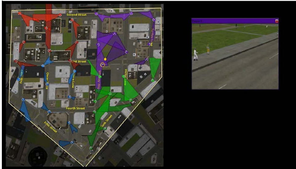
Figure 1. Screen capture of the multi-sensor management interface (MSMI) providing the Full North-Up Map display (left) and the video feed of a single camera (right).
