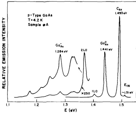
FIG. 1.  $T = 4.2$ -K PL characteristics of a  $p$ -type sample (sample A). The near-intrinsic region emission ( $E_{in}$ ),  $C_{As}$ -related emission at 1.493 eV and the emissions at 1.441 and 1.284 eV due to  $Ga_{As}^0$  and  $Ga_{As}^-$ , respectively, are seen.
