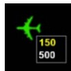
Figure 2. Aircraft icon and data block showing airspeed (150 kts) and altitude (FL (flight level) 500)
