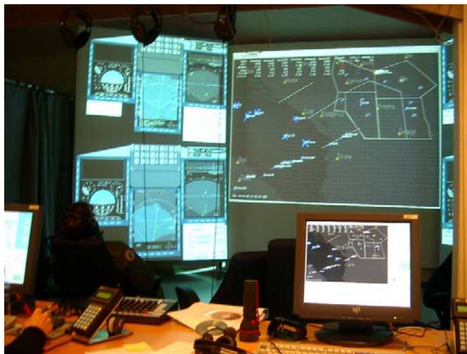
Figure 1. The FLSC instructor and operator station, and in the background the debriefing facilities using the old scenario visualization tool.
