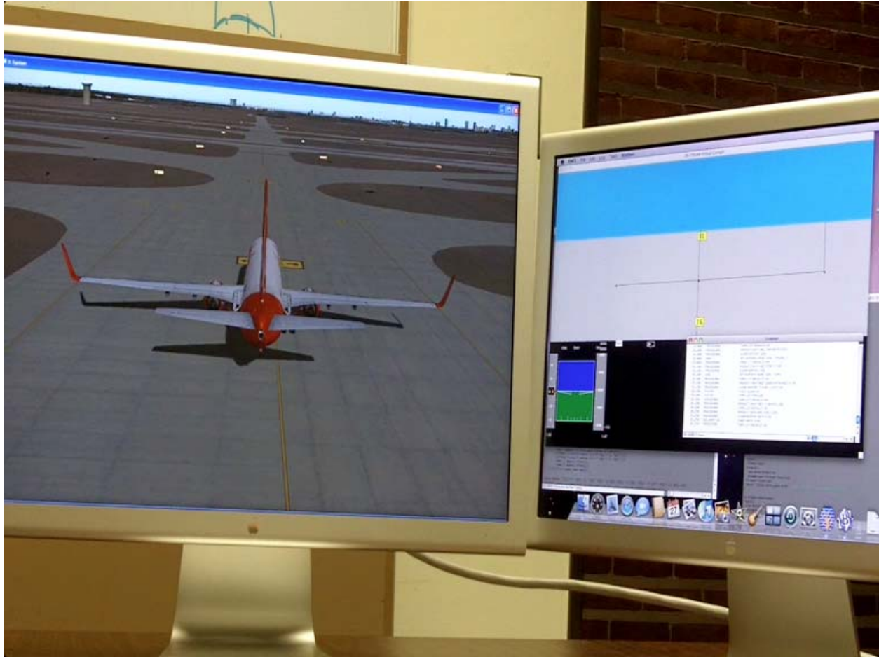
Figure 2. X-Plane is shown on the left monitor, and the virtual cockpit and ACT-R trace are shown on the right monitor.
