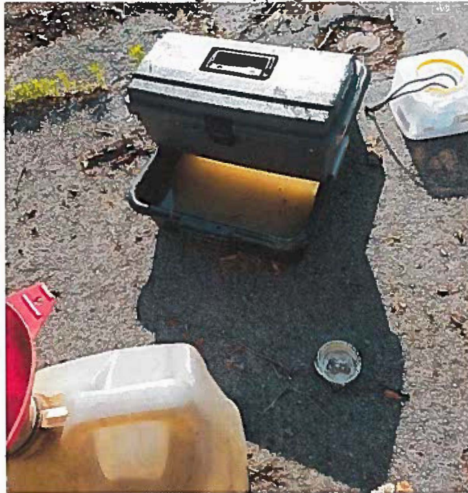
Figure 1: Fully constructed Gravid Trap, complete with mosquito brew lure. The pictured trap is ready to be placed in its location for overnight trapping.
