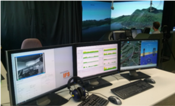
Figure 4. Workplace of the flight instructor with three display elements. Left: operator console, center: resource monitor, right: cockpit displays
