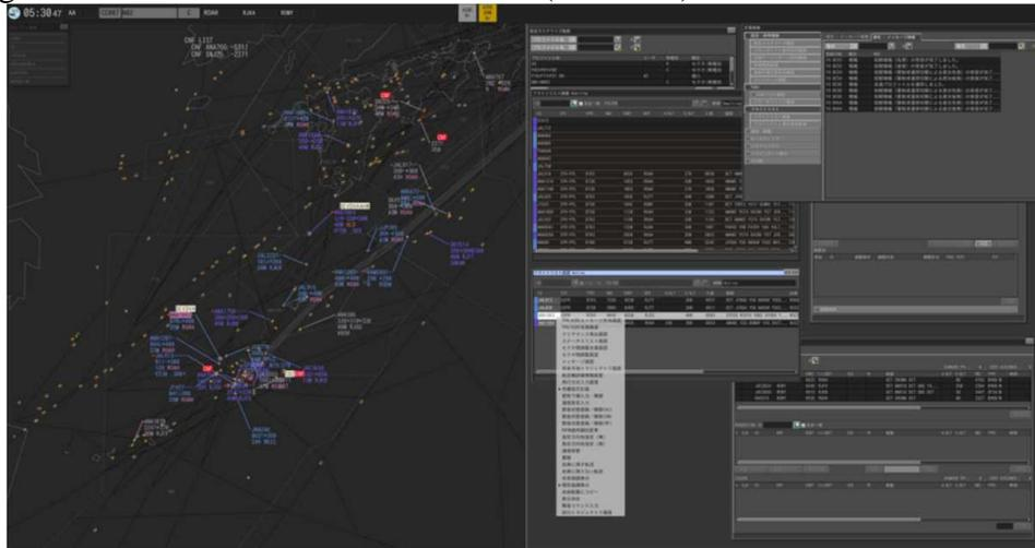
*Figure 1.* An example of TEPS main display. Left side shows the radar domain and the other side is support domain. The position information served by air route surveillance radar combined with flight planning information. (Ministry of Land, Infrastructure, Transport and Tourism, Overview of TEPS, Retrieved from <https://www.mlit.go.jp/koku/content/001358999.pdf> (In Japanese))
