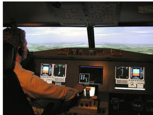
**Figure 1.** MITRE Air Traffic Management Lab Cockpit Simulator
