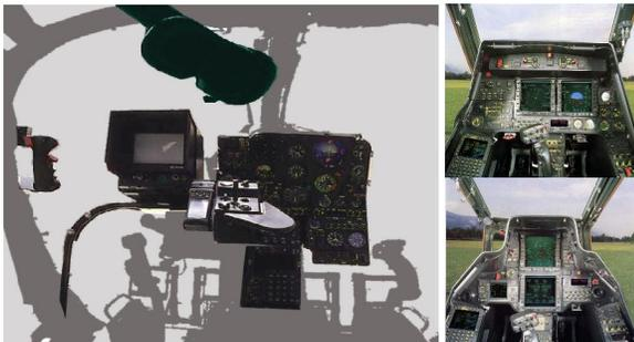
**Figure 1.** Left Viviane Gazelle, Right Tigre front (top) and back seat (bottom). The technological leap between former and later helicopter HMI is tremendous. Notice the numerous multiple function display (MFD) in the Tigre cockpit.
