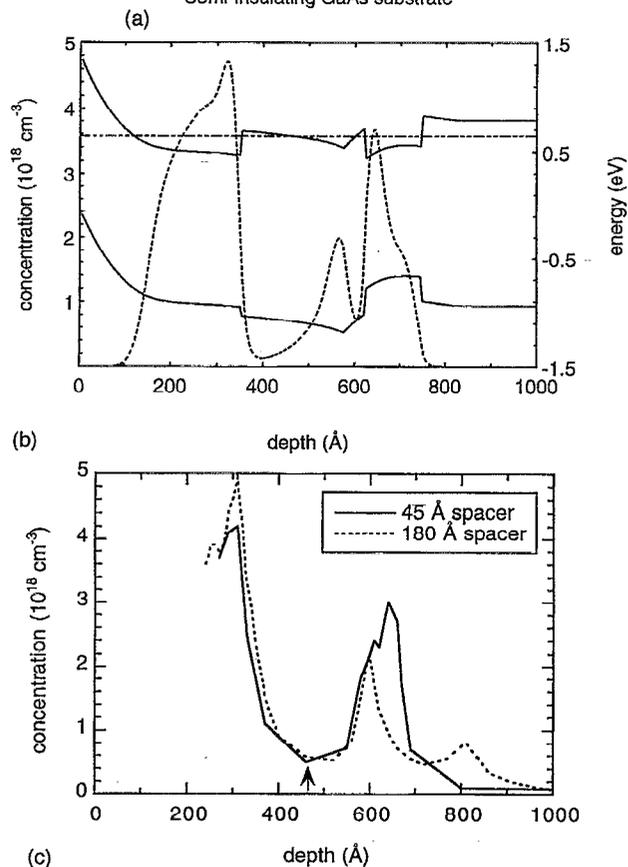
FIG. 1. pHEMT with a 45 Å spacer: (a) layer structure; (b) theoretical calculation showing the energy bands (solid line), the carrier concentration (dashed line), and the Fermi level (chain line); (c)  $EC-V$  measurement with an arrow showing where integration begins.
