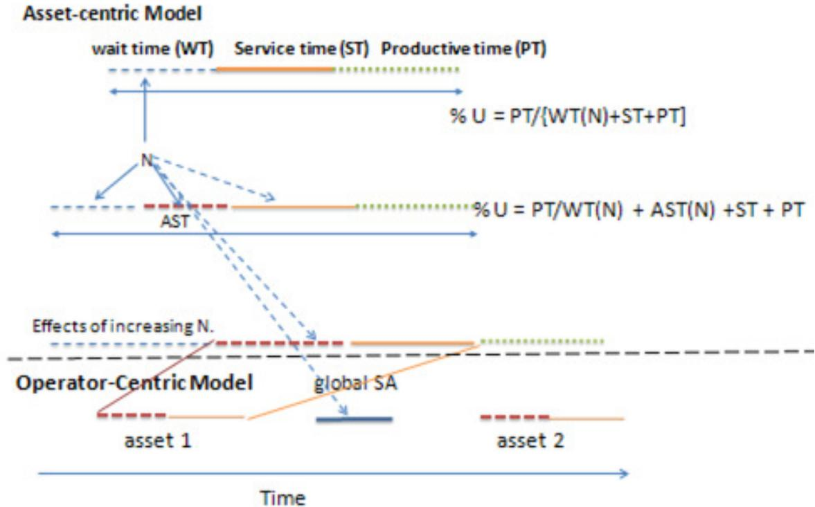
**Figure 2.** Components of the time cycle for each asset. The influence of  $N$  on these components is shown by comparing the second and third time line, where it can be seen that in the third time line the percent Utilization (productive time to total time) is diminished. On the bottom the foundations of the operator-centric model are depicted, showing the servicing of two assets and the time required to maintain global SA (the solid line).
