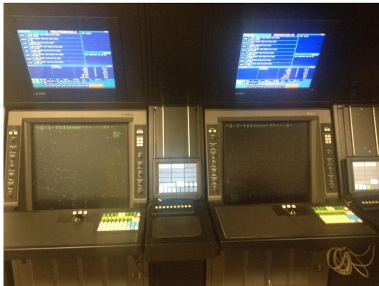
Figure 1. Air Traffic Control Specialist (ATCS) workstations in the Research Development and Human Factors Laboratory (RDHFL).
