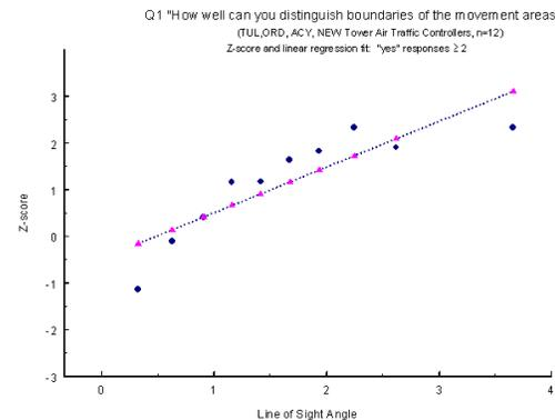
**Figure 4.** Converting the proportion of “yes” responses for response 2 or greater to Z scores, and then fitting a linear line showed that 50% of the observers reported 0.481 degrees as the preferred line of sight angle of incidence.
