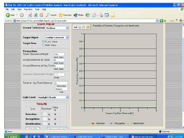
**Figure 1.** Object discrimination tool graphical user interface. Users enter tower height and distance to calculate air traffic control tower specialists' detection and recognition of an airport surface object.
