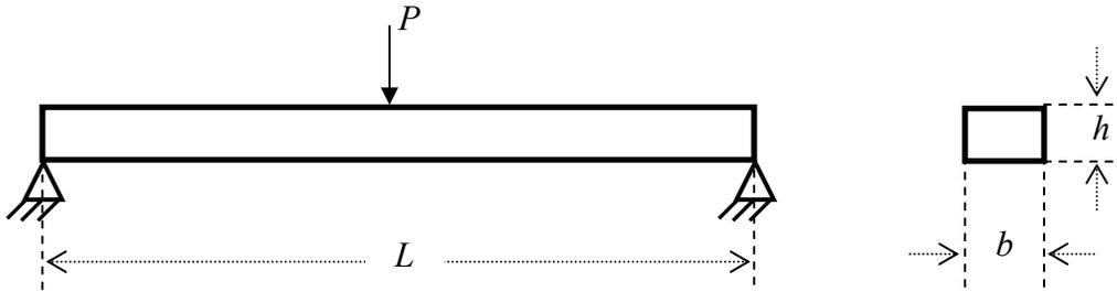
**Figure 5.2:** Simply Supported Beam
