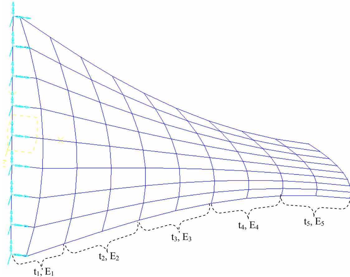
**Figure 4.3:** Finite element model of the turbine blade
