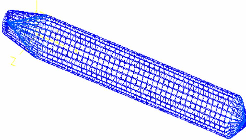
**Figure 3.9:** Finite Element Model of a Torpedo Hull
