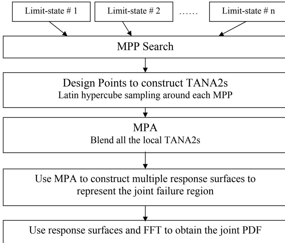
**Figure 3.4:** Algorithm Details for System Reliability Estimation
