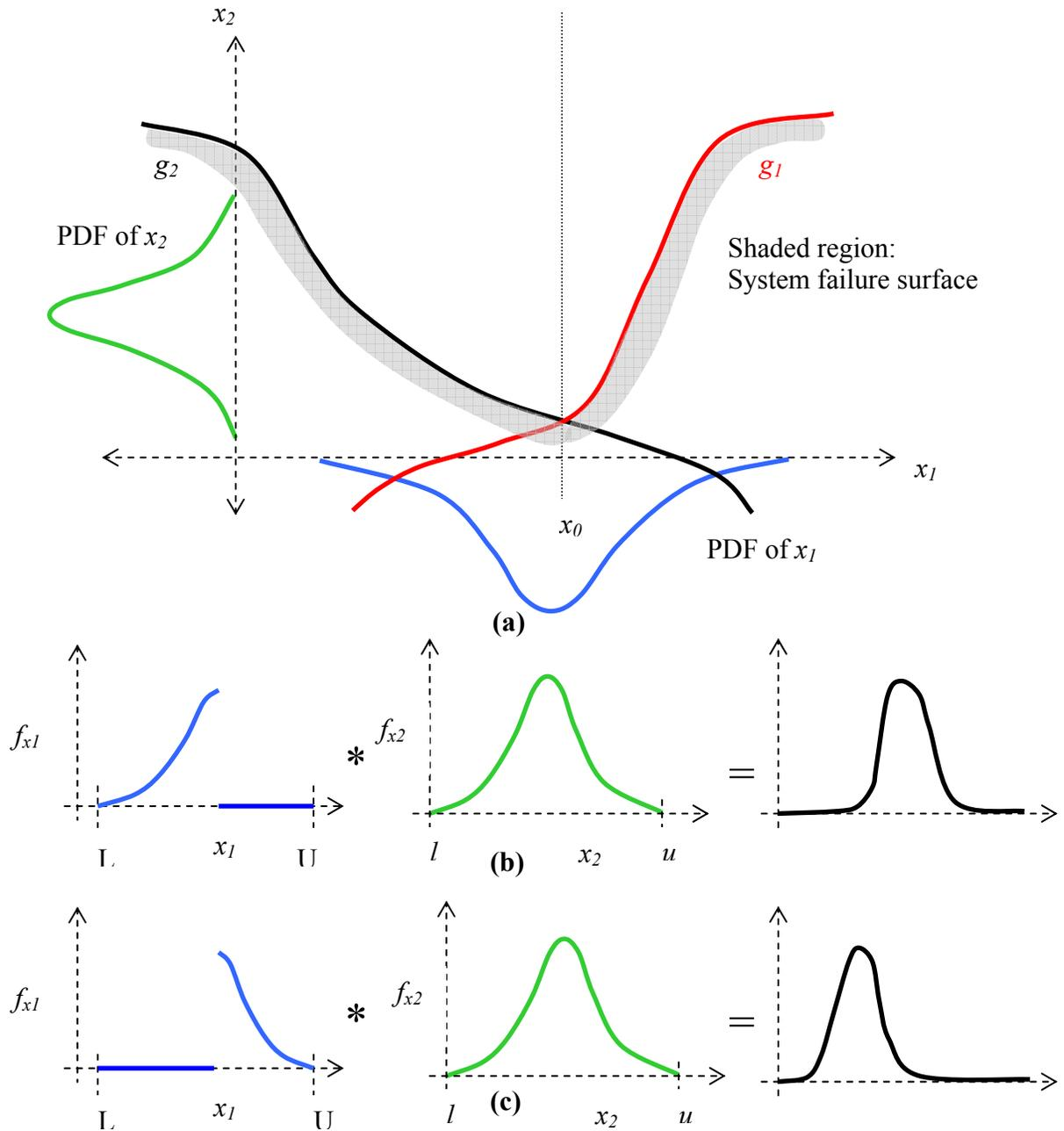
**Figure 3.1:** Convolution Based on More Than One Function
