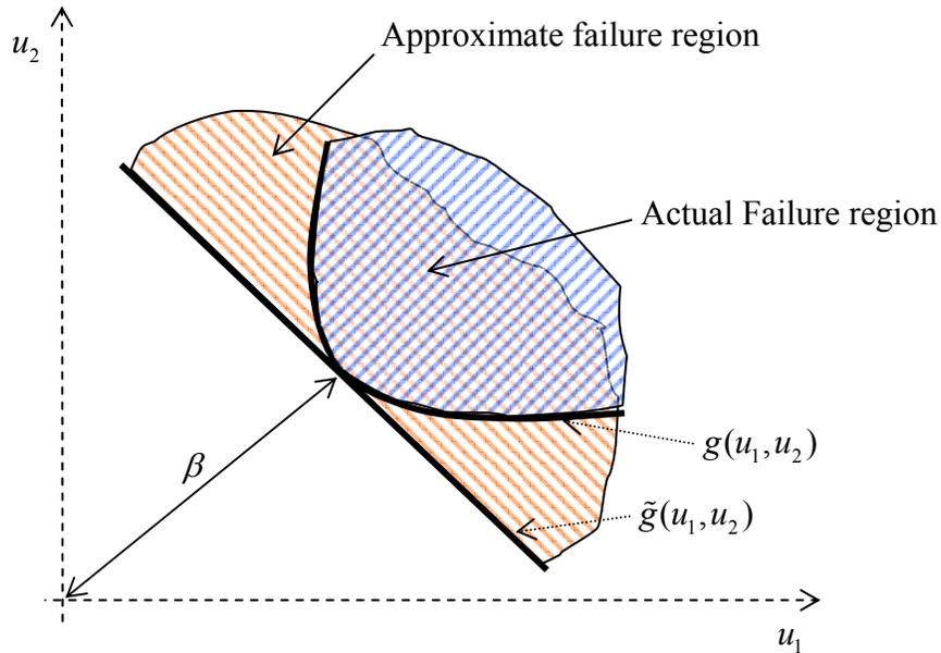
**Figure 1.6:** Failure Surface Based on Safety Index
