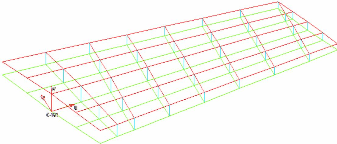
**Figure 2.12:** Finite Element Model of the Wing Structure
