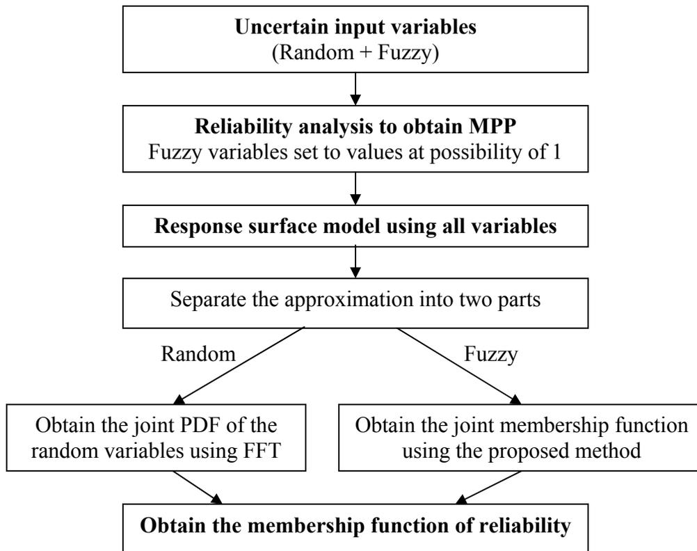
**Figure 2.6:** Algorithm for Estimating Membership Function of Reliability
