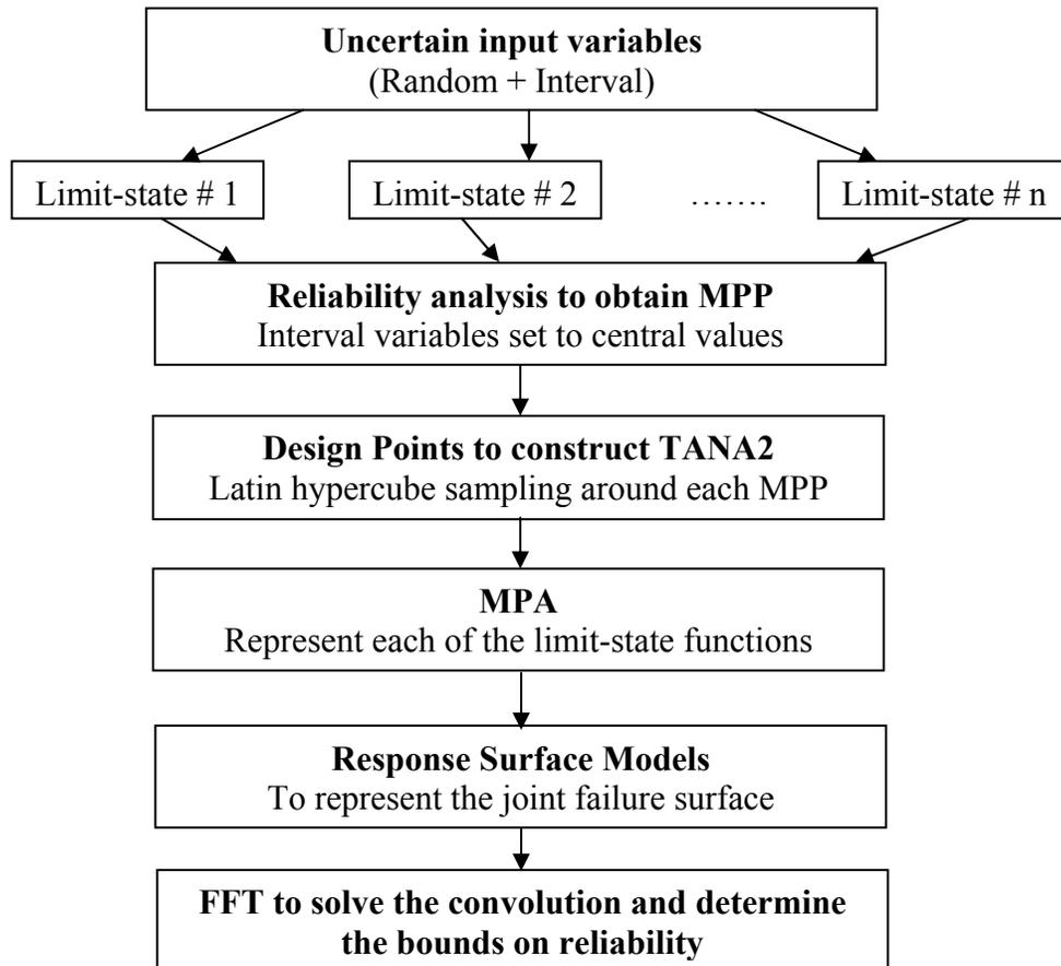
**Figure 4.1:** Methodology for Estimating System Reliability Bounds
