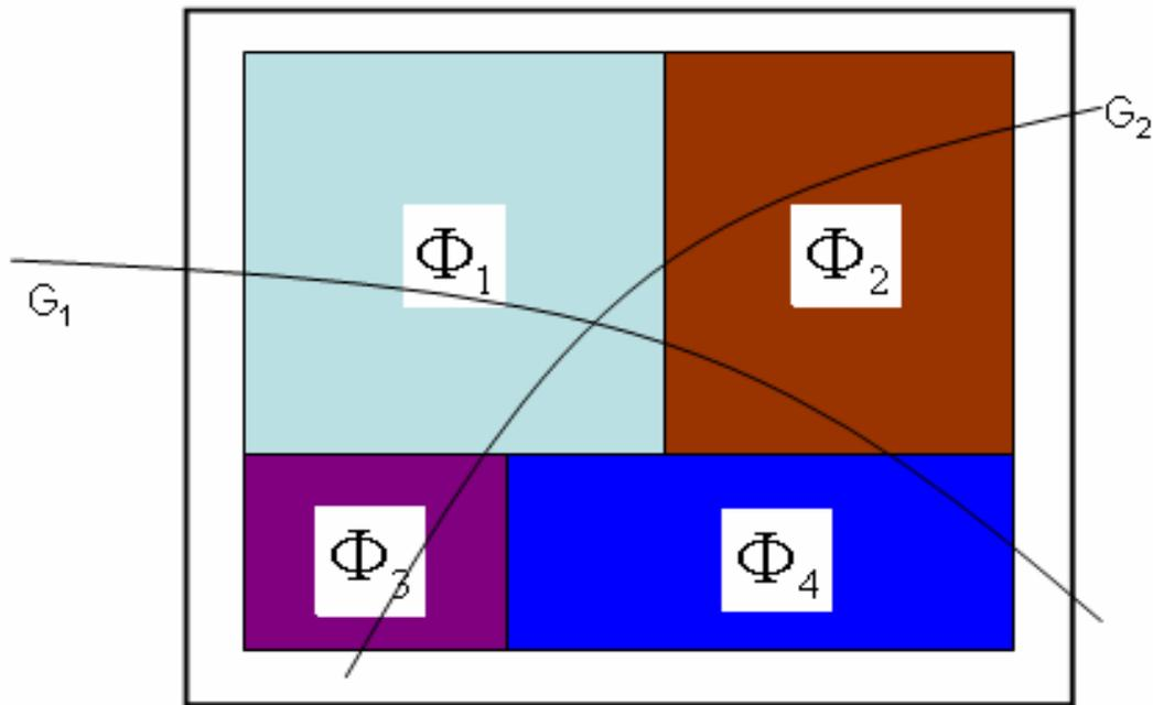
**Figure 3.2:** Solving the Convolution Integral in Intervals
