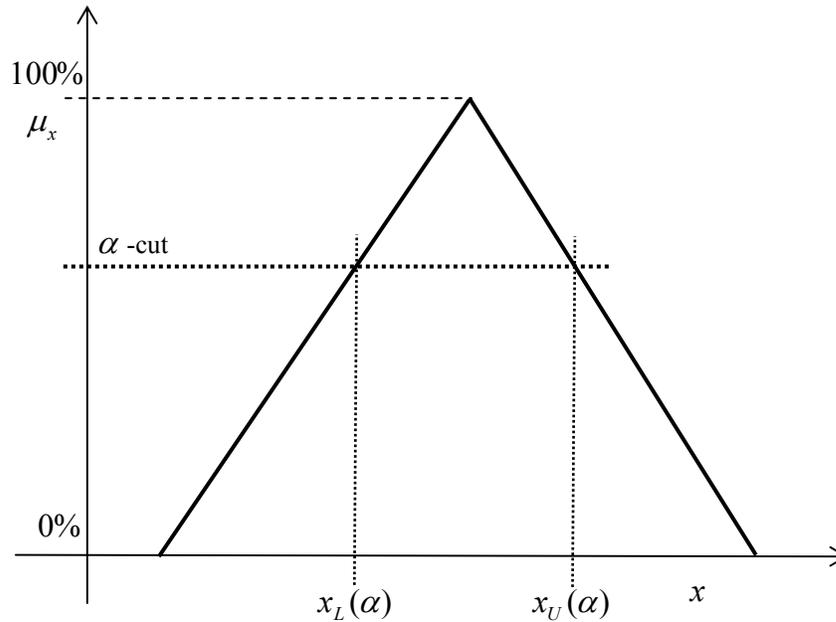
**Figure 1.5:** Membership Function Showing an  $\alpha$ -cut
