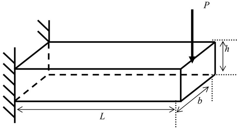
**Figure 3.6:** Cantilever Beam
