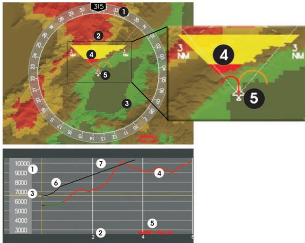
Figure 1: EGPWS display layout: HSD (top) and VSD (bottom) presentation.
