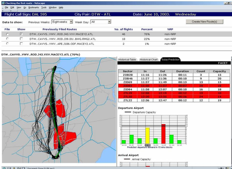
**Figure 5.** Tabular presentation of FACET sector data, graphical display of FACET data on traffic demand at arrival and departure airports, and map display of FACET data and filed (green) vs. flown (black) routes. (The red sectors on the map represent sectors with “high” traffic volume.)
