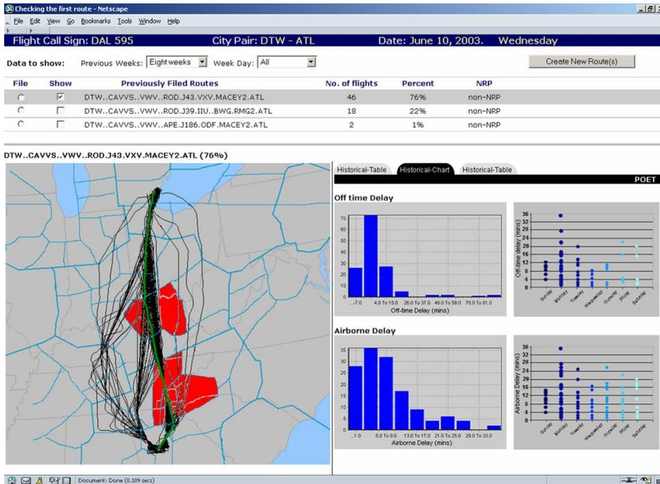
**Figure 4.** Graphical presentation of historical flight performance data along with map display of FACET data and filed (green) vs. flown (black) routes. (The red sectors on the map represent sectors with “high” traffic volume.)
