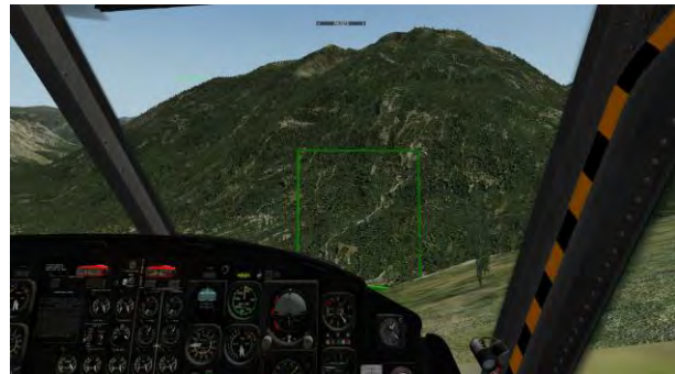
Figure 1 . Gates define the target flight path in the primary flight task. Ideally, participants fly from the center of one gate to the center of a subsequent gate.
