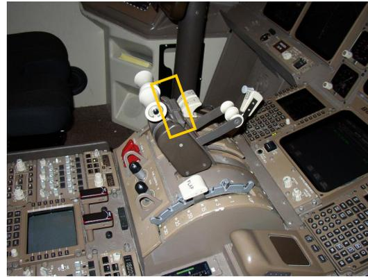
**Figure 1.** Boeing 777 throttle quadrant with TOGA switch highlighted.
