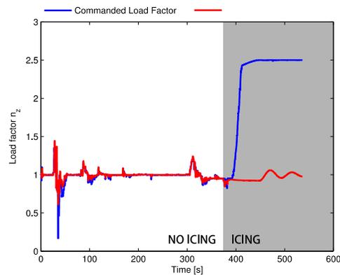
Figure 8. Example of commanded and measured load factor.
