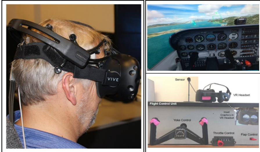
Figure II. The configuration of the HTC Vive virtual reality headset and EMOTIV EPOC+ EEG headset on the left. The participants' view of the simulation environment is displayed on the top right, and the physical instrument layout is shown on the bottom right.
