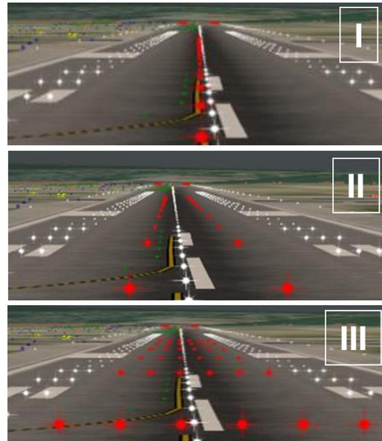
**Figure 5.** Alternative THL Lighting Configurations for Study 2
