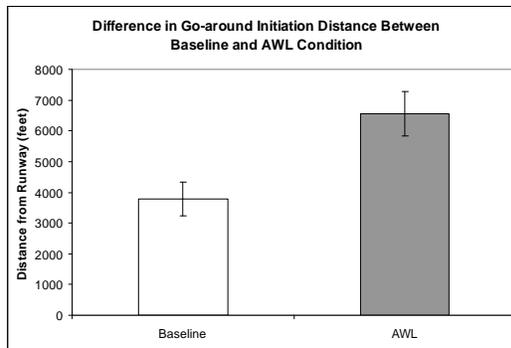
**Figure 7.** Difference in Go-around Initiation as Response to Arrival Warning Lights (AWL) Versus Baseline Condition
