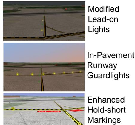
**Figure 1.** Passive Warnings Included Airport Surface Markings and Lightings
