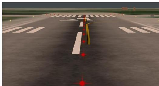
**Figure 6.** Simulation Representation of Runway Remaining Lights
