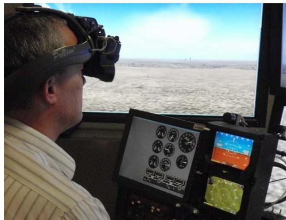
Participants wore a Kaiser (now Rockwell) Optical stereoscopic full-color see-through HMD (640 by 480 resolution; 25% transmissivity; Figure 1). The display was head-position slaved so that obstructions generated in the HMD overlaid obstructions visible in the out-the-window scene.
