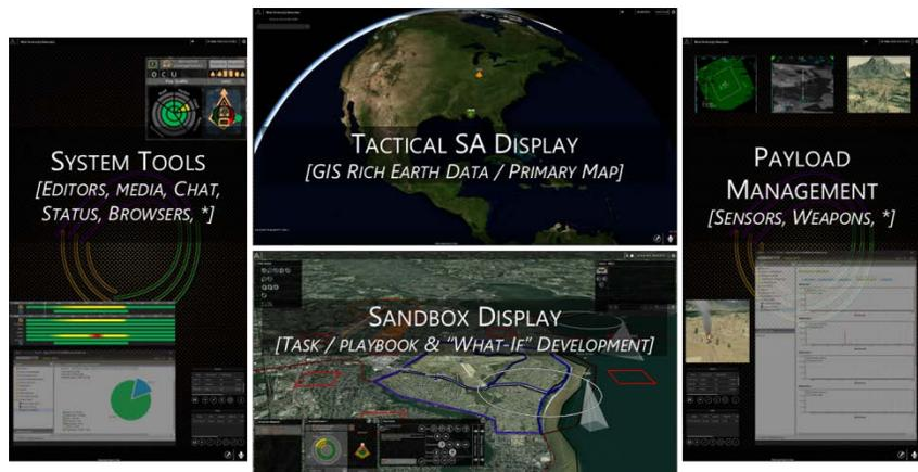
The IMPACT instantiation of Fusion, as shown in Figure 5, employs a four screen layout: system tools, real time tactical situation awareness (SA) display, sandbox tactical SA display, and sensor management. The operator uses the sandbox display to perform all of their play calling and chat monitoring tasks. The other screens display tools to enhance the operator’s SA.
