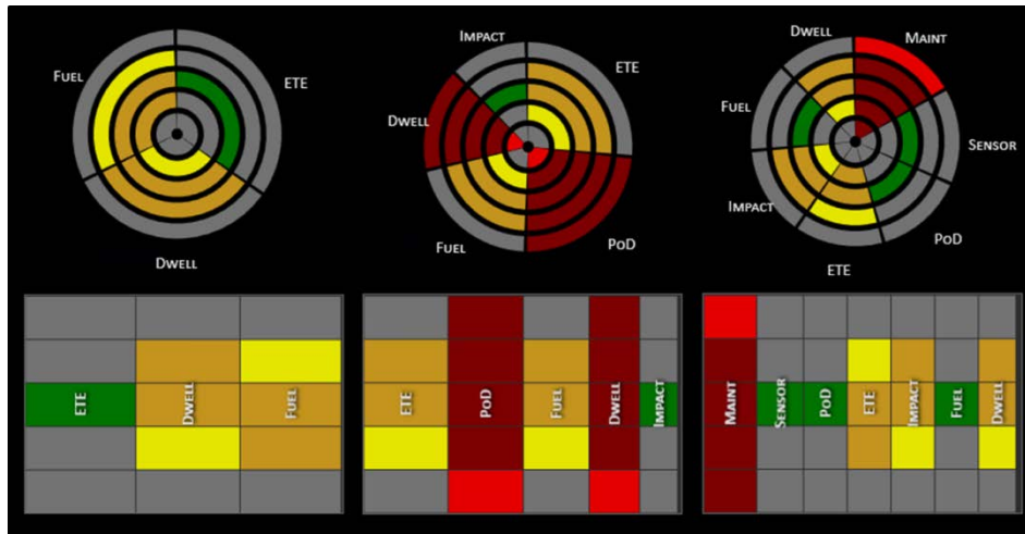
Figure 2. Sample Pie and Bar Chart Formats depicting three, five, and seven parameters of unmanned vehicle plan status. Each chart was approximately 2 X 3 in.
