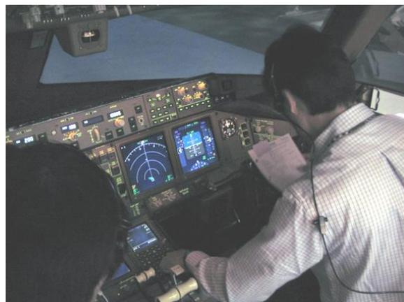
**Figure 1.** Entering the flight data into the FMC: the pilot reads aloud the information on the paper while inputting the data
