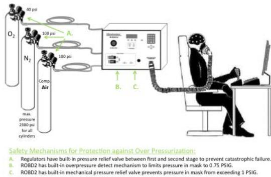
Figure 1. Schematic depiction of ROBD-2 configuration
