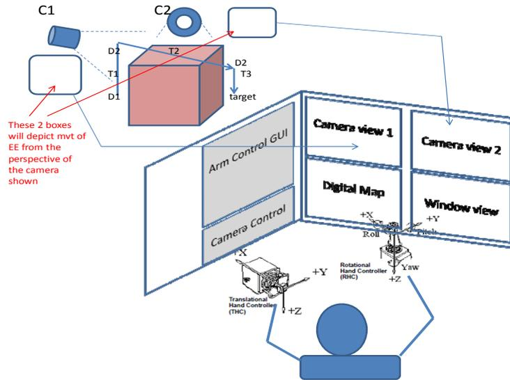
**Figure 1.** Schematic description of the robotic arm workspace (upper left) and displays. The figure depicts only two (rather than 6) camera views (C1 & C2) and a window view, and, within the workspace, a typical mission, to move the EE up, across a table and down to a target.
