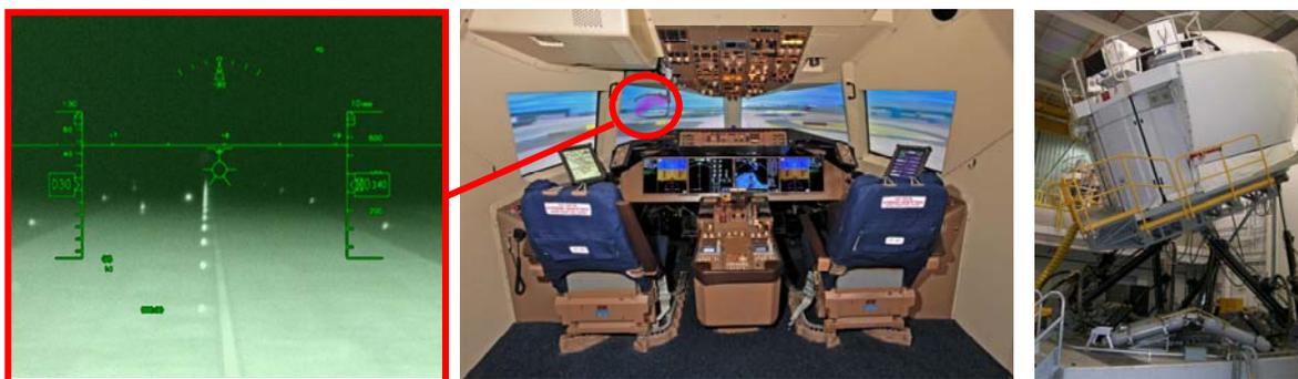
**Figure 2. Full Motion-Based Commercial Aircraft Simulator (Enhanced Vision HUD shown)**
