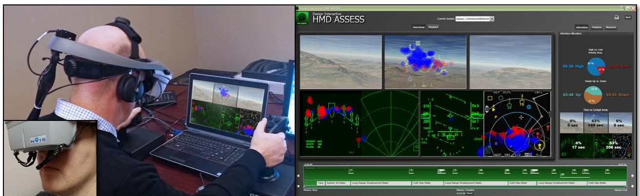
Figure 1. HMD ASSESS Prototype (left) and Instructor Displays (right) with notional iconography and data for the purposes of the paper.
