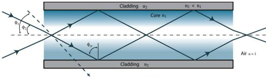
Fig. 6. Standard optical fiber light path. There is a slight refraction as the light enters the fiber from air. Cladding is used with a different index of refraction ( $n_2$ ) to minimize light from escaping and entering. Based on the critical angle  $\Phi_{cr}$ , the light either refracts into the cladding barrier or reflects back into the core as related to the angles of incidence  $\Phi_1$  and  $\Phi_2$ .
