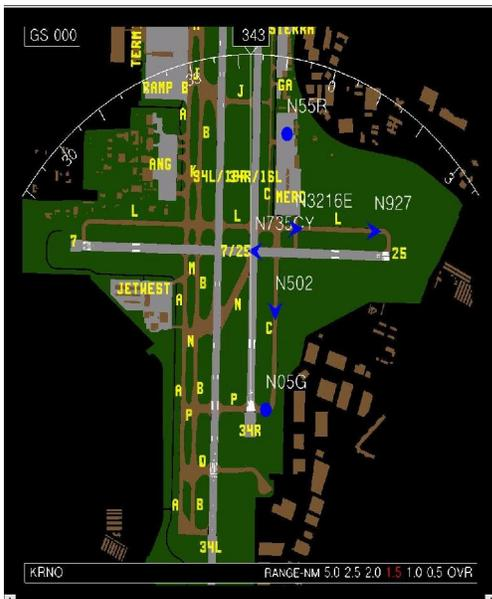
Figure 3. Plan-View Surface Map with Traffic (BMOT)
