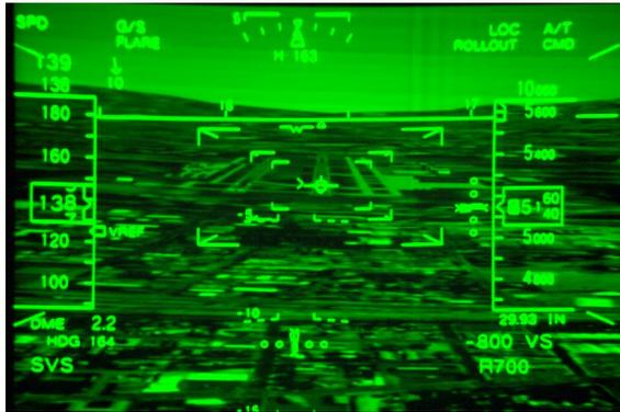
Figure 1. Fused HUD Concept with Tunnel
