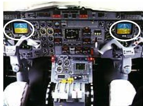
Figure 2. EMB120 Brasília panel with both Flight Directors (FD) – <http://www.airliners.net> (authorized by L. Ten Hoppen)
