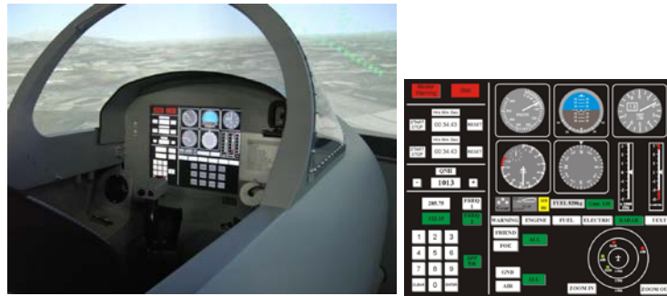
Figure 1. The flight simulator used in Phase III/ fixed wing (FPS/F) consists of cockpits with a high quality screen comprising the field of view (200° horizontal, 45° vertical) (left), and the multifunctional display showing expanded instrumentation as well as touchscreen and radio (right).
